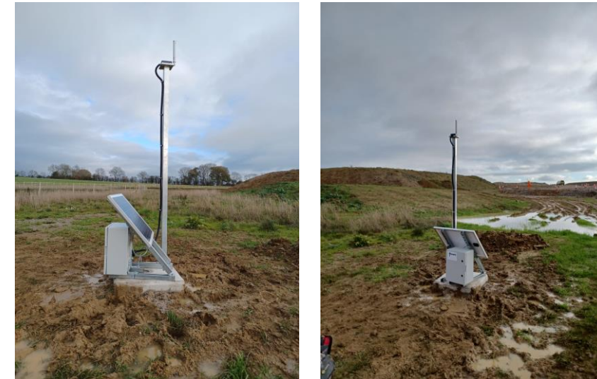
Fig 2. Measurement setup of GeoCubes in the field.
